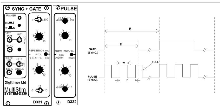
The D331 module allows the user to set the **Repetition Interval (R)** and **Gate Duration (D)** independently. The pulse **Frequency (f)** and **Width (w)** are both controlled by the D332 module.
