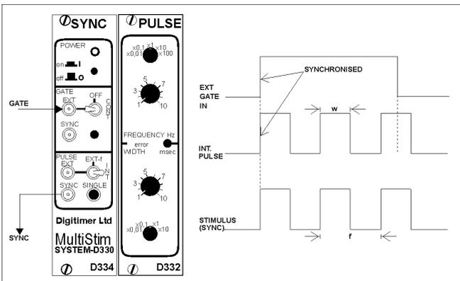
Here the **Width (w)** and **Frequency (f)** are being controlled internally by the D332. Note that Pulse 1 starts synchronously with the start of the **Gate** 'opening'. Note also that, since pulse 3 starts **before** the **Gate** 'closes', the whole pulse is delivered to the preparation.
