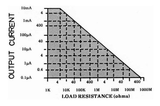
Fig. NL800A-2 Graph showing the Current that can be delivered dependant on the load Resistance. Currents can be delivered to loads within the hatched area.
