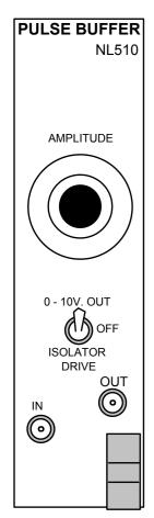
The **NL510 PULSE BUFFER** converts TTL logic pulses into either pulses whose amplitude can be set to between 0 and 10V pulses or input drive pulses for the **NL800 Stimulus Isolator**.
