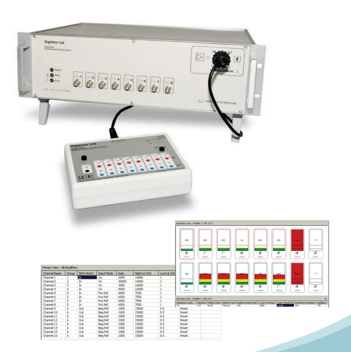
Electrode impedance checking allows the D360 operator to instantly identify electrodes exhibiting unacceptable resistances. Impedance levels are indicated by green, yellow and red bars within the Impedance View Window (right), or by eight tri-colour LEDs visible on the electrode connection headbox. The resistance values at which the colours change can be custom set by the operator.
