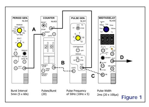
sends a regular output pulse at the interval set on the front panel. This output resets and activates the **NL603 COUNTER**, sending it's output at (B) "high" until the count reaches the preset value of 20.
