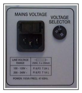
Changing the mains voltage will also require you to change the two fuses in the mains inlet. They must be "5 x 20 mm" in size and the value and speed shown here.
