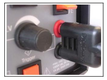
More force is required to fully insert the connector.
