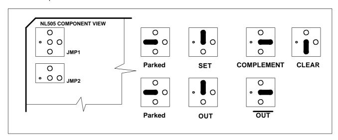
The on-board jumpers allow a single connections between adjacent modules without the need of external cables. The position of these jumpers are changed by gently pulling them away from the PCB, then rotating them 90°, 180° or 270° before replacing them in two of the small gold board sockets.
