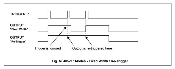
In **FIXED WIDTH** mode, the NL405 will produce an Output pulse of the duration as specified on the Front Panel regardless of further Trigger applied to the input (IN). Trigger pulses received during the time the Output (OUT) is active are ignored.
