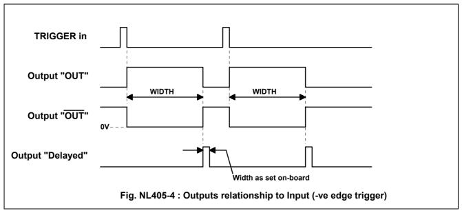
The above two figures show the effect of selecting "+ve edge" or "-ve edge" triggering.
