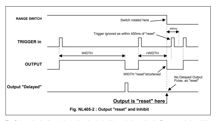
The Output pulse duration can be terminated early, in either mode, by rotating the Range control. It would be normal, in this instance, to rotate it to the next 'click' position and then back to where it was set. The Outputs are inhibited for 450 ms after the switch becomes still. Note that a Delayed Output pulse is NOT generated at the end of a WIDTH that is terminated early.
