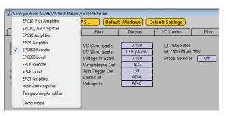
When in Remote mode, the controls and knobs of the EPC 800 USB are inactive. All amplifier settings are fully controlled by PATCHMASTER. The mode of operation is set from within the Configuration / Hardware window of PATCHMASTER.
