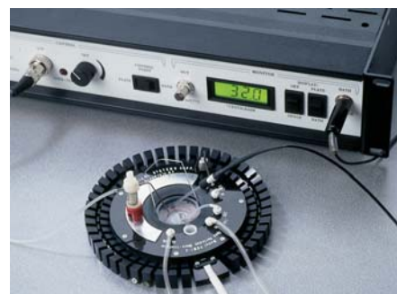
The PDMI-2 and TC202A provide a temperature controlled environment for 35mm dishes
